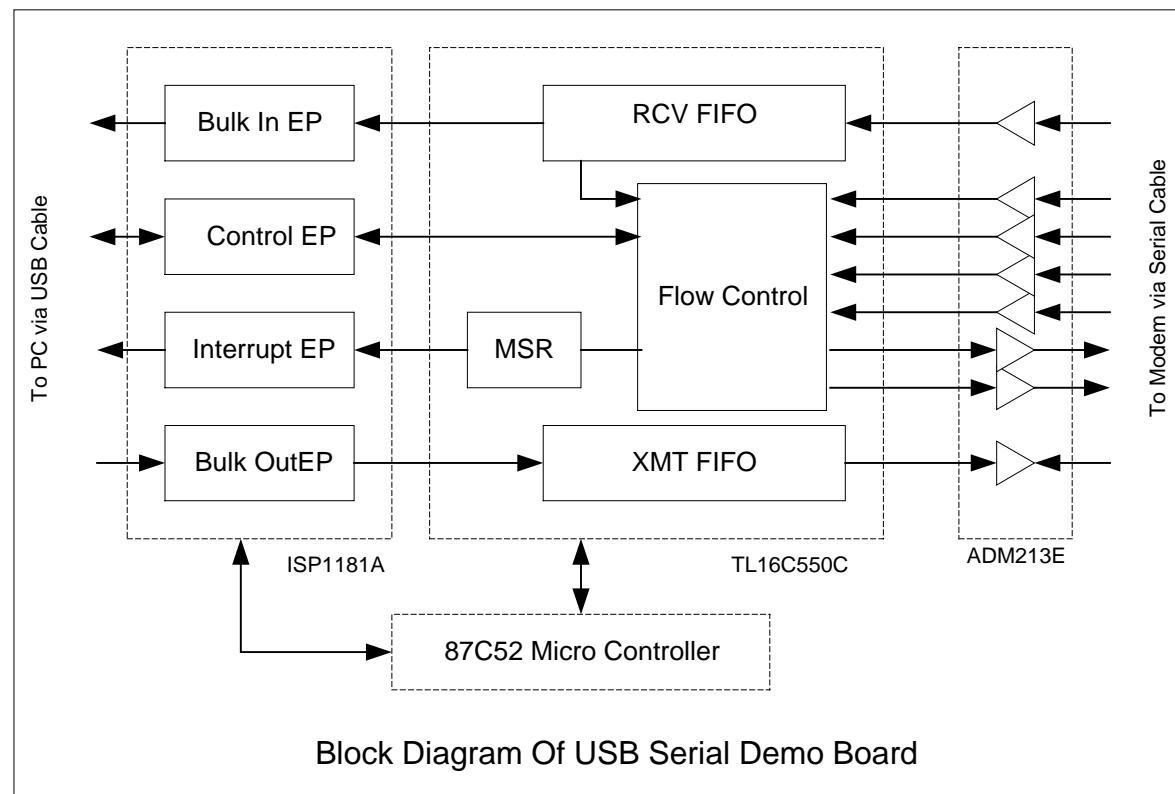
The ISP1181x is a full-speed, cost-optimized and feature-optimized USB interface device with up to 14 configurable endpoints. It has a high-speed general-purpose parallel interface for communication with many kinds of microcontrollers or microprocessors. It supports different bus configurations and local DMA transfers of up to 16 bytes per cycle.
